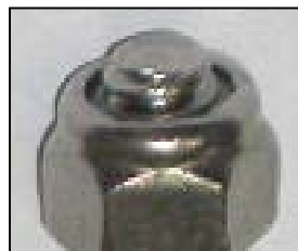
Figure 2. Incorrect - too tight. Screw extends beyond edge of nut.
