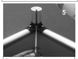
Place rubber caps on legs and insert legs into bottom corner. Rotate leg so slot aligns with set screw hole. Secure in place with set screw. This is purposely a tight fit so it will take some effort to fully tighten screws.
