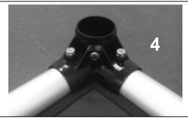
Place a bottom corner bracket over pipes, insert bolts through openings, secure with lock washers and hex nuts and hand tighten. Insert and secure second bolt. Repeat process at each of other three corners.
