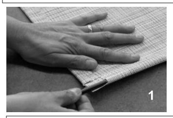
Lay fabric flat with underside facing up and insert cording into sleeve. Note that 40oz Vinyl fabric comes with cording in the sleeve.
