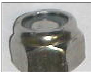
Figure 1. Correctly tightened. Screw is flush with nylon locking material
