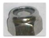
DO Correctly tightened. nut is flush with bolt
