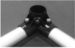
4. Position one bottom corner on the top half of the frame and guide bolt ends through the bottom corner holes. Secure each bolt with a washer and nut but do not tighten all the way. Repeat process on further 3 corners.
