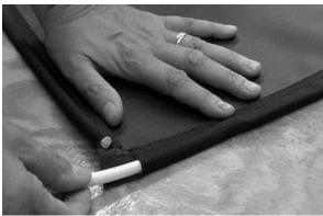
1. Lay fabric flat with underside facing upwards. When using the ballistic nylon fabric you are required to manually slot the cording into the fabric sleeves. This step is not required for the 40oz vinyl fabric as the cording is already encased into the vinyl sleeves.
